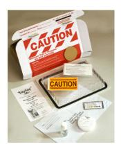
Testing for moisture using a Calcium Chloride test kit (ASTM F 1869 Standard Test Method for Measuring Vapour Emission Rate of Concrete Subfloor Using Anhydrous Calcium Chloride) will require 3 tests for the first 1,000 sq. ft. and at least one additional test for each 1,000 sq. ft. thereafter. Maximum allowable reading shall be 3 lbs. per 1,000 sq. ft. **Contact StaticWorx for Calcium Chloride Test**
