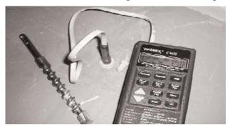
Testing for moisture using a Humidity Probe and Digital Meter (ASTM F 2170 Standard Test Method for Determining Relative Humidity in Concrete Floor Slabs Using in situ Probes) will require 3 tests for the first 1,000 sq. ft., and at least one additional test for each 1,000 sq. ft. thereafter. Maximum allowable reading shall be 75% RH.
