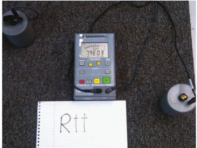
Measuring resistance between points (RTT) on an 'ESD-grade' carpet tile using two NFPA probes. (Note extreme low resistance 7.9 \text{ E } 03 = 7900 ohms. NFPA 99 minimum resistance is 25,000 ohms.)
